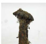
Distorted deflector plate
