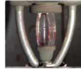
Called strutting, when exposed to heat the glass does not shatter correctly, holding the seal in place and so stopping the water from being released.
