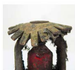
Distorted deflector plate
