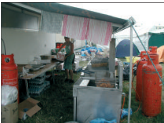
Figure 13: Mobile deep fat fryers too close to combustibles
